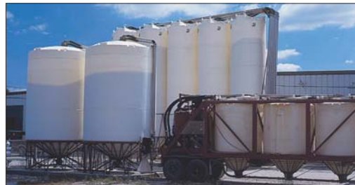
Large cone bottom tanks ranging in sizes from 2,500 to 13,000 gallons, are used to store and deliver up to 10,000 cubic ft. of bulk resins at a processing plant.
